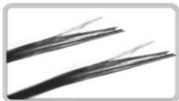
Hundreds of fibers are pulled together to form single weave strands of Kevlar®.
