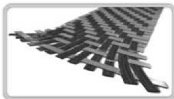
Strands are woven together to make up different patterns; the woven patterns are then dipped to create a malleable material.
