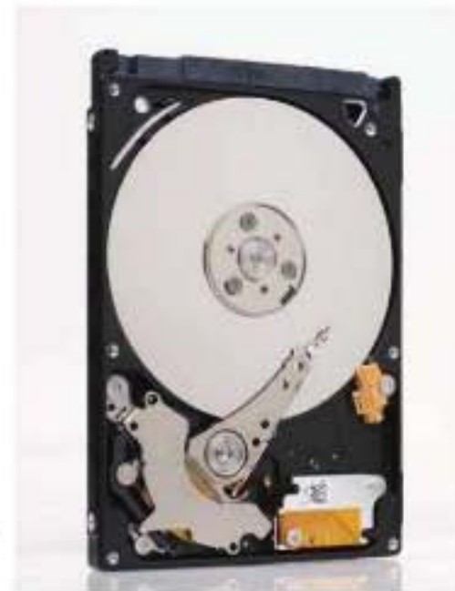
above: Under the hood. Internal hard drives are constantly being reinvented – the Momentus Thin from Seagate is just 7mm thick.
